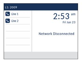
Check that the cables are tightly connected to the phone and to the wall jack. The phone should automatically detect when it is reconnected and remove the **Network Disconnected** promptfrom the screen. However, if changes have been made to your phone's network settings, you may need to restart your phone. Check with your System or Network Administrator for assistance.
