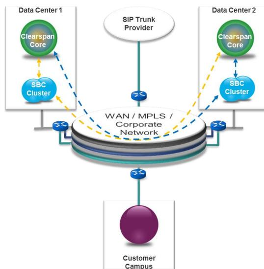
**Figure 12. SBC Cross Coupling.**
