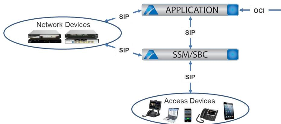
**Figure 4. CORE SBC Platform Interaction.**
