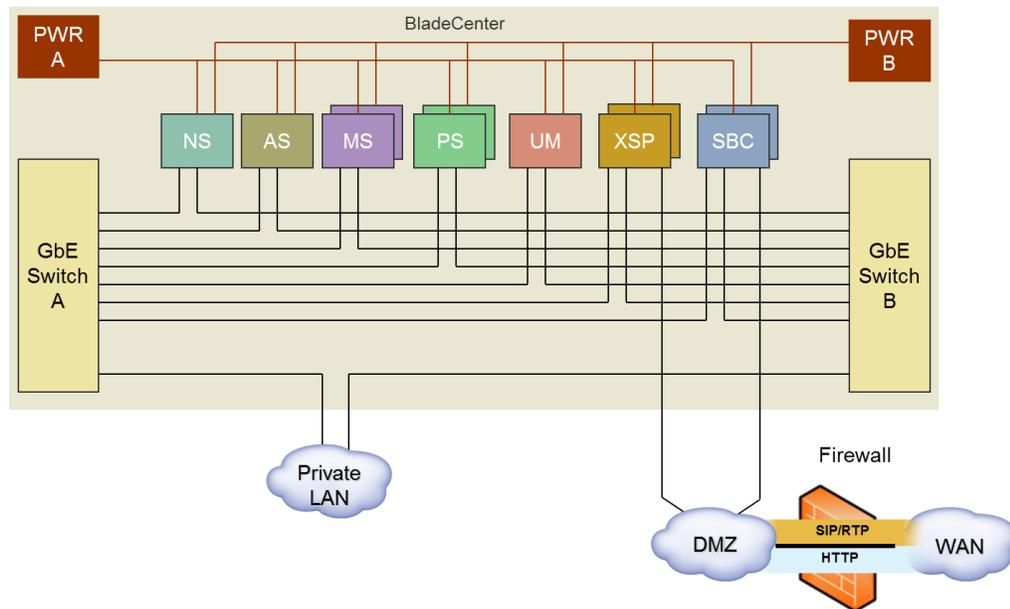
**Figure 11. Typical High-level BladeCenter Architecture.**
