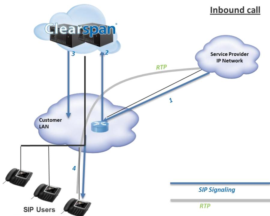
**Figure 17. Clearspan Inbound Signaling and Call Flows.**
