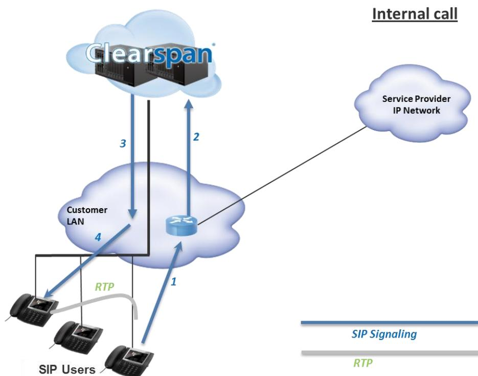
**Figure 19. Clearspan Internal Signaling and Call Flows.**
