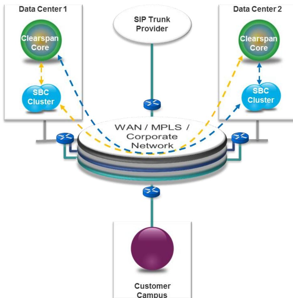
**Figure 1. High-Level Clearspan Architecture.**
