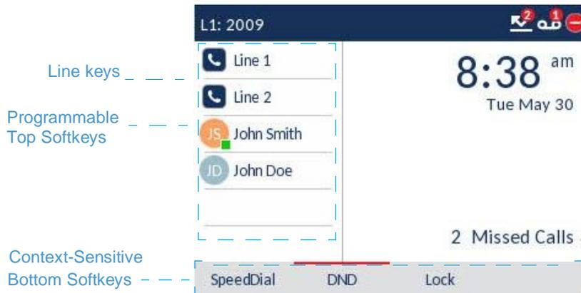
The state-sensitive softkeys change depending on the state of the phone and are used to perform different functions when the phone is in an idle, connected, outgoing, or busy state.
