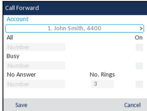
2. Press the left and right navigation keys to change to the desired account.
