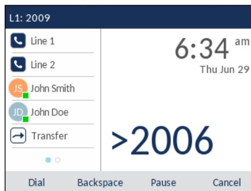
With the phone in an idle state and on-hook, simply use the dialpad to enter the number you wish to call, and after reviewing the number, press the **Dial** softkey. Use the **Backspace** softkey to correct any errors and the **Pause** softkey to insert pauses.
