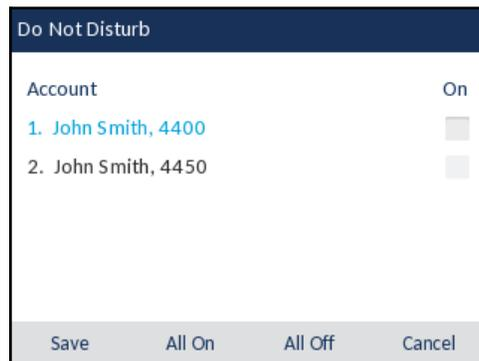
2. Use the up and down navigation keys to scroll through the accounts and press the select button to enable DND for the selected account.
