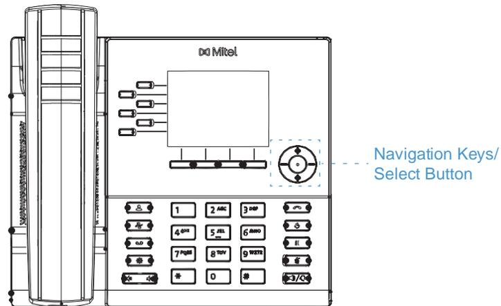
There are four directional keys (up, down, left, and right) on the navigation cluster that can be used to navigate through the various applications and settings menus. The center key acts as a **Select** button that is used to set options and perform actions such as dialing out from the **Contacts** or **Call History** applications.
