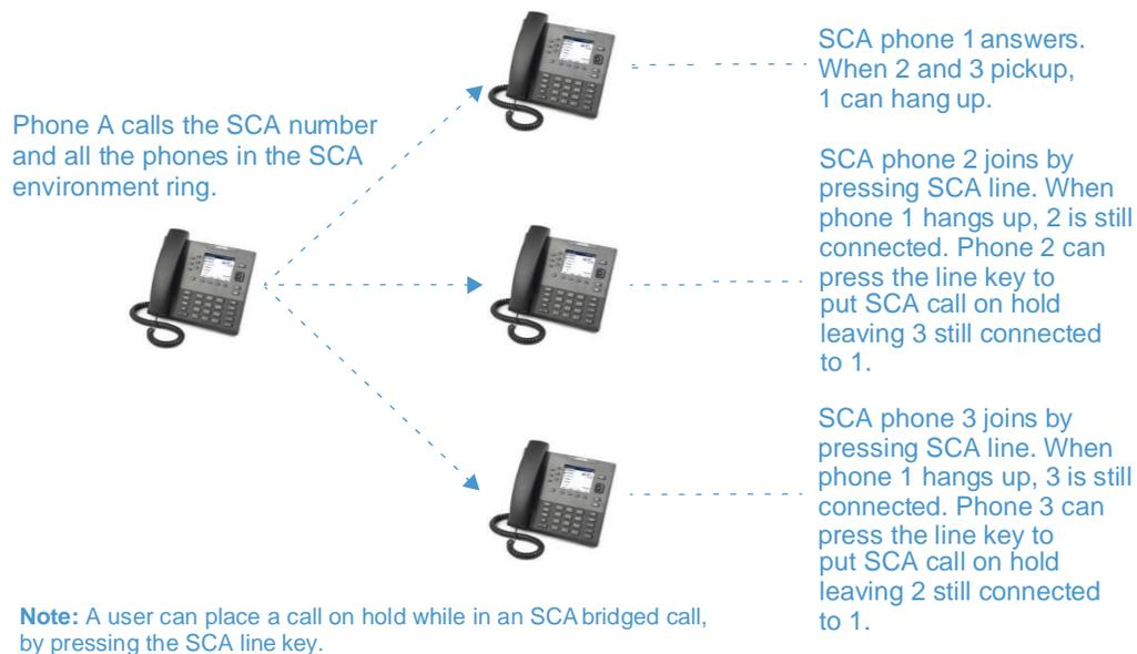
Using the example above, when a call comes into Phone 1, Phone 2 and Phone 3 can pickup the same call by pressing the SCA line key. Phone 2 and 3 display the call they are bridging into on the LCD of the phones. Existing SCA parties in a bridge or one-to-one call hear an audible beep when another party has joined the call.
