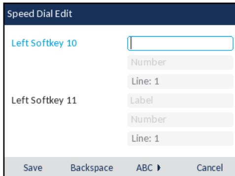
4. Navigate to the desired key and in the **Label** field (if applicable), enter a label to apply to the key.
