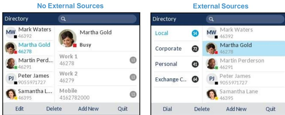
(Optional) If the contact has multiple phone numbers defined, press the **▶** key to navigate to the numbers selection column (if no external Directory sources are configured/enabled) or Details page and use the **▲** and **▼** keys to select the desired phone number.
