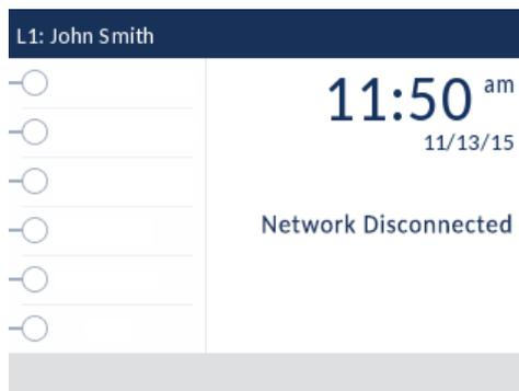
Check that the cables are tightly connected to the phone and to the wall jack. The phone should automatically detect when it is reconnected and remove the **Network Disconnected** prompt from the screen. However, if changes have been made to your phone's network settings, you may need to restart your phone. Check with your System or Network Administrator for assistance.
