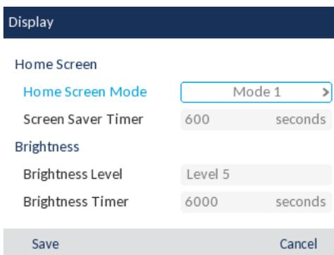
3. Use the ◀ and ▶ navigation buttons to increase or decrease the intensity of brightness on the LCD.
