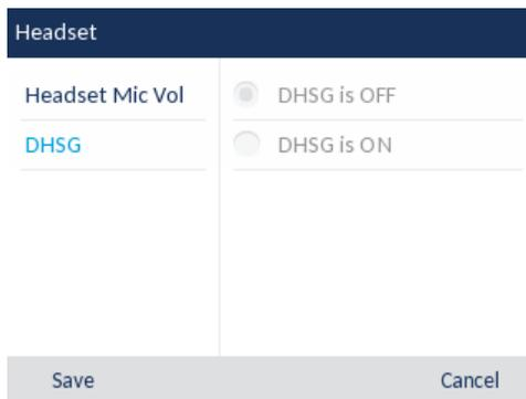
6. With **DHSG** highlighted press the **▶** key to move to selection column.
