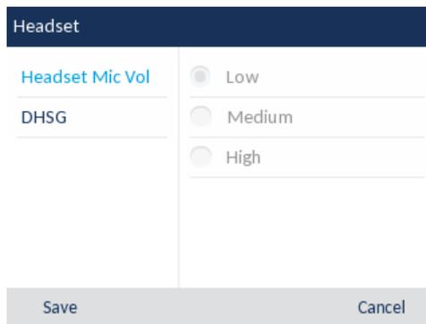
3. With **Headset Mic Vol** highlighted press the **▶** key to move to selection column.
