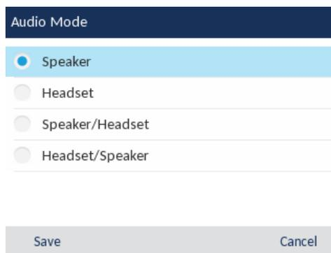
3. Use the ▲ and ▼ keys to scroll through and highlight the desired audio mode. Valid values are:
