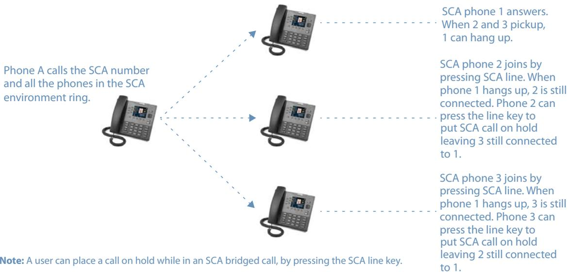
Using the example above, when a call comes into Phone 1, Phone 2 and Phone 3 can pickup the same call by pressing the SCA line key. Phone 2 and 3 display the call they are bridging into on the LCD of the phones. Existing SCA parties in a bridge or one-to-one call hear an audible beep when another party has joined the call.
