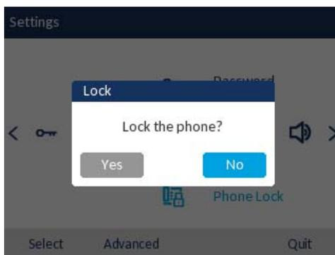
3. At the **Lock the phone?** prompt, press the **Lock** softkey or navigate to the **Yes** button and press the
